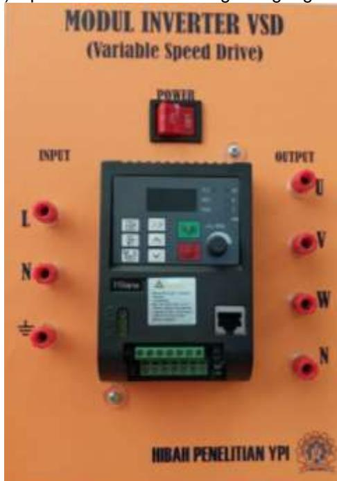
**Gambar 7.** Modul Inverter Variable Speed Drive.
