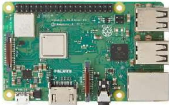
Gambar 3. Raspberry Pi 3 Model B+.
